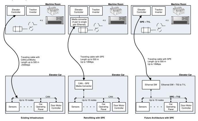
**Elevator Car-to-Machine Room Communication**
