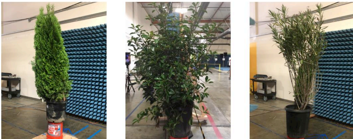
Figure 10: Three foliage types evaluated in penetration experiments: (a) Dense Foliage (White Cedar), (b) Medium-Density Foliage (Photinia), (c) Sparse Foliage (Oleander)
