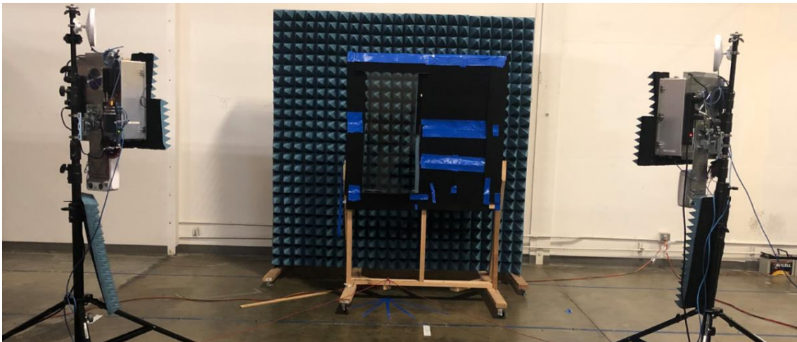
Figure 12: Photograph of measurement setup for reflection through Glass #1. Non-glass reflective surfaces and the backside of the glass are covered with an RF absorbent foam to prevent reflections from other materials
